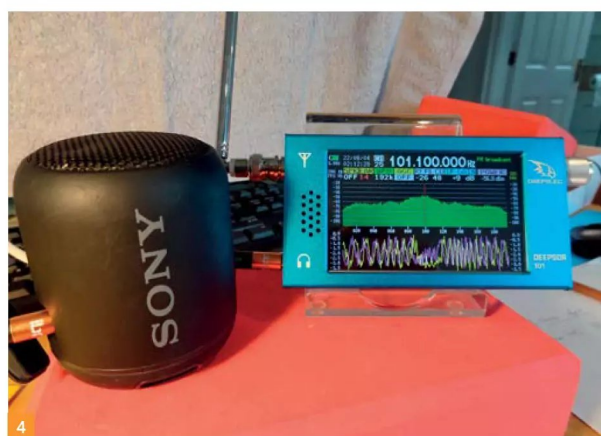
Fig. 1: Out of the box: the DeepElec Deep SDR 101. Fig. 2: Block diagram for the DeepElec Deep SDR 101. Fig. 3: Tap away here: the frequency direct-input screen. Fig. 4: Enhance the sound by connecting an active speaker. Fig. 5: RAF VOLMET on 5,450kHz coming in on the telescopic.
